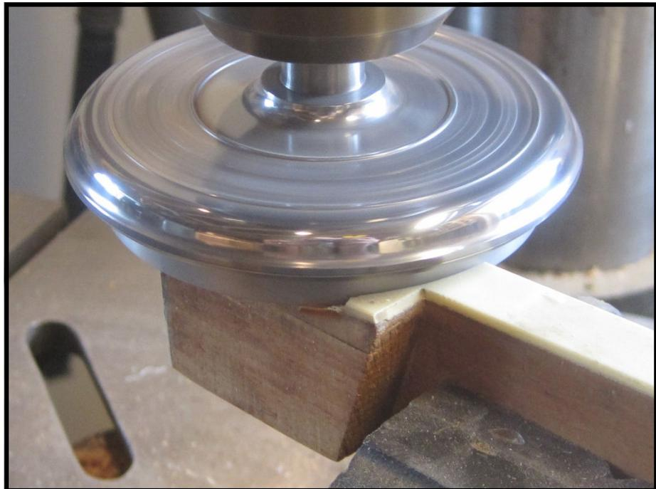
to compensate for the greater thickness of the new keytop material. This milling down process gives a completely flat surface on which to glue the new keytops.
