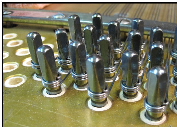
New tuning pins and strings being installed.
