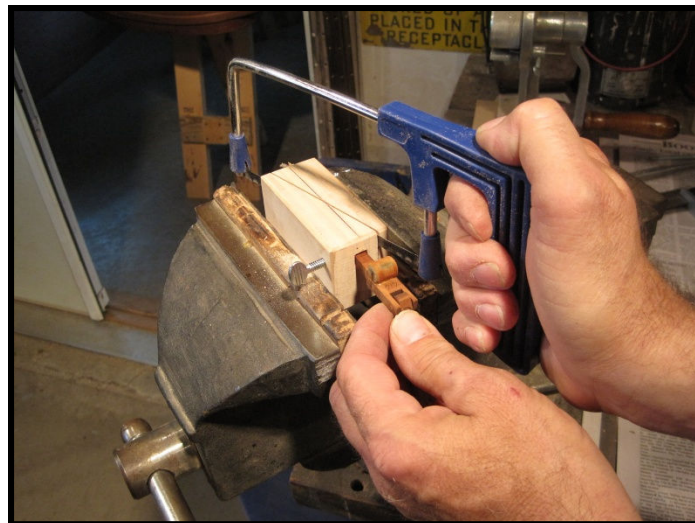
Special sawing jig required.
